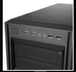
Front I/O: 2x USB 3.0, 2x USB 2.0, 2x audio
