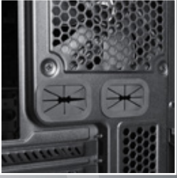
2x Openings for water cooling
