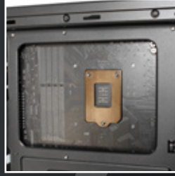
Installation opening for CPU coolers
