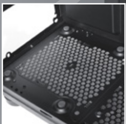
PSU decouplers and dust filters
