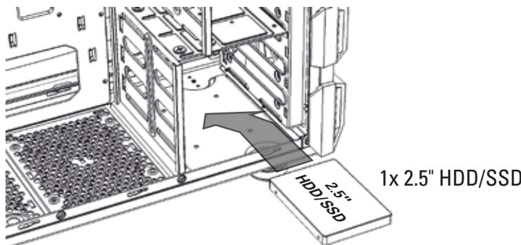
**EN** Installation of a 2.5" HDD/SSD (screw type)
